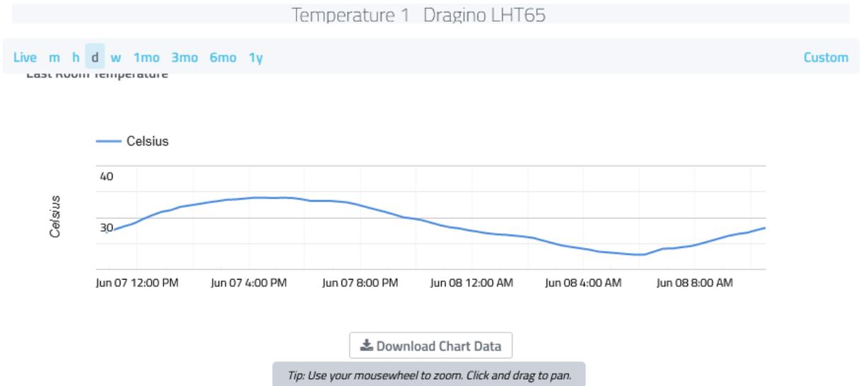
Figure 3. Diurnal temperature readings in the east room of the onsite swine farm. The data was retrieved from the Cayenne user interface (dashboard). Note the “Download Chart Data” button that allows one to save historical records as an Excel file.
