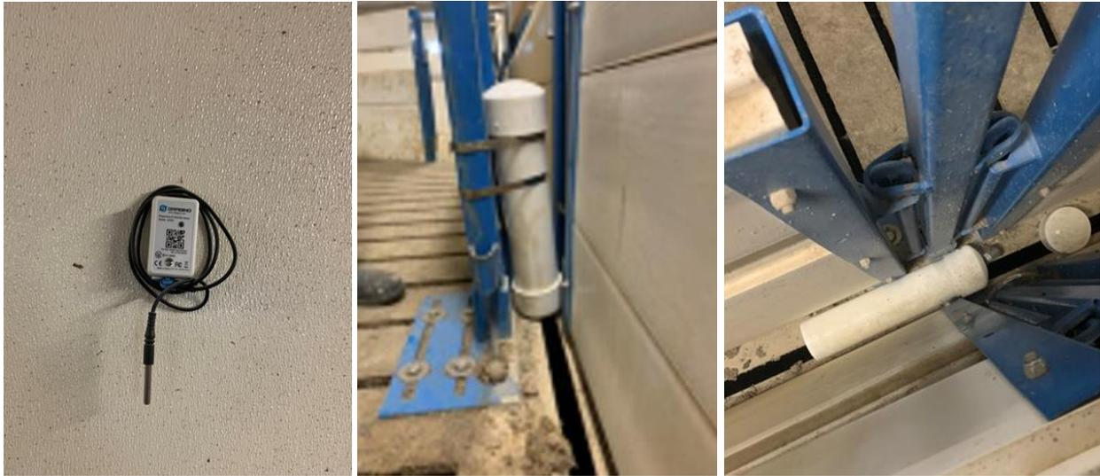
Figure 1. (Left) Installation of the LHT65 temperature/humidity sensor. One can see a heavy-duty temperature probe on an extension cable; (Middle) Installation of the LDDS75 ultrasonic distance sensor with a PVC shield; (Right) The LDDS75 sensor being tipped over by pigs.
