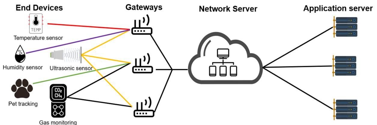
Figure 1. LoRaWAN monitoring system architecture
